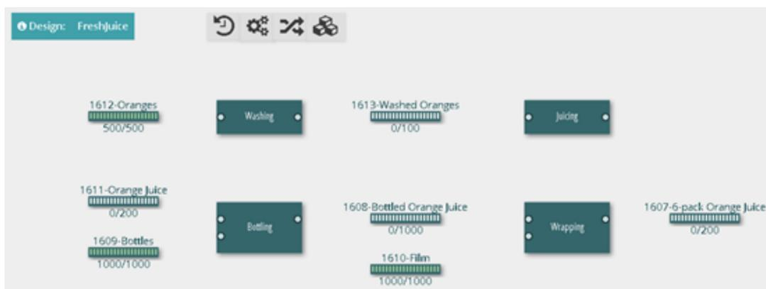
b) Next, the characteristics of the inputs and outputs of each Machine must be determined and the connections between the Machines and the Carriers should be made. The circles on the left side of each Machine are connections for inputs, while those on the right side are output connections.
