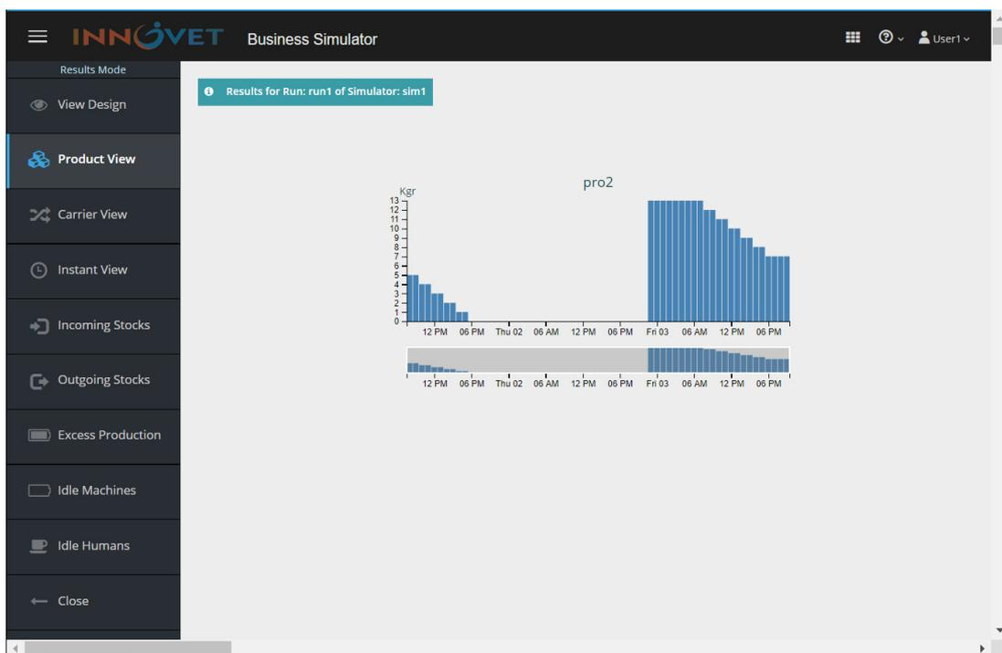
In the environment of the system, a graphical representation of the product *pro2* quantities, appears. The vertical axis represents the product quantity and the horizontal axis represents the simulation time. The user is able to select the displayed time span by adjusting accordingly the dynamic frame situated under the graph.
