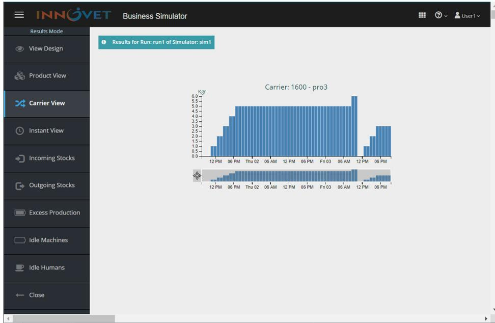
In the environment of the system, a graphical representation of the product *pro3* quantities transferred by the Carrier 1600, appears. The vertical axis represents the product quantity and the horizontal axis represents the simulation time. The user is able to select the displayed time span by adjusting accordingly the dynamic frame situated under the graph.
