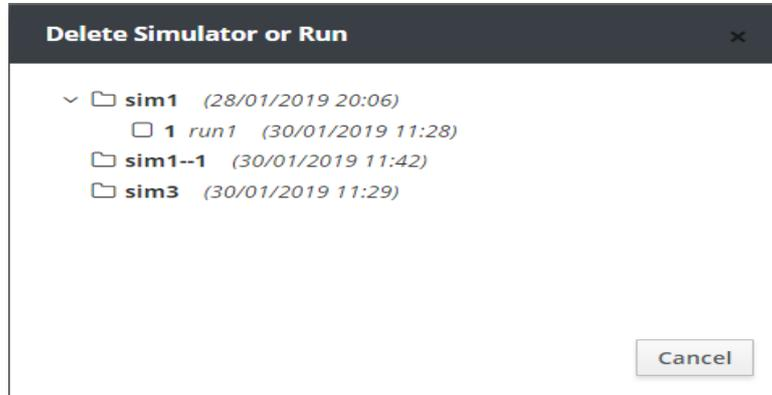
① Select the Simulator *sim1--1*. The following window appears, warning the user that the preceding Simulator will be deleted.
